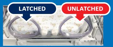
You must pull on the **bedside panel** every time the panel is closed to make sure that the panel is latched.
