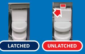
You must pull on the **bedside panel** every time the panel is closed to make sure that the panel is latched.
